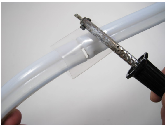
Figure 9: Shrink the tube by heater for each Connected portion
